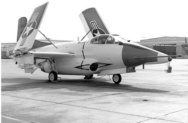
The Shrike test platform was a TF-10B aircraft fitted with an A-4E nose section in place of the regular bulbous nose
