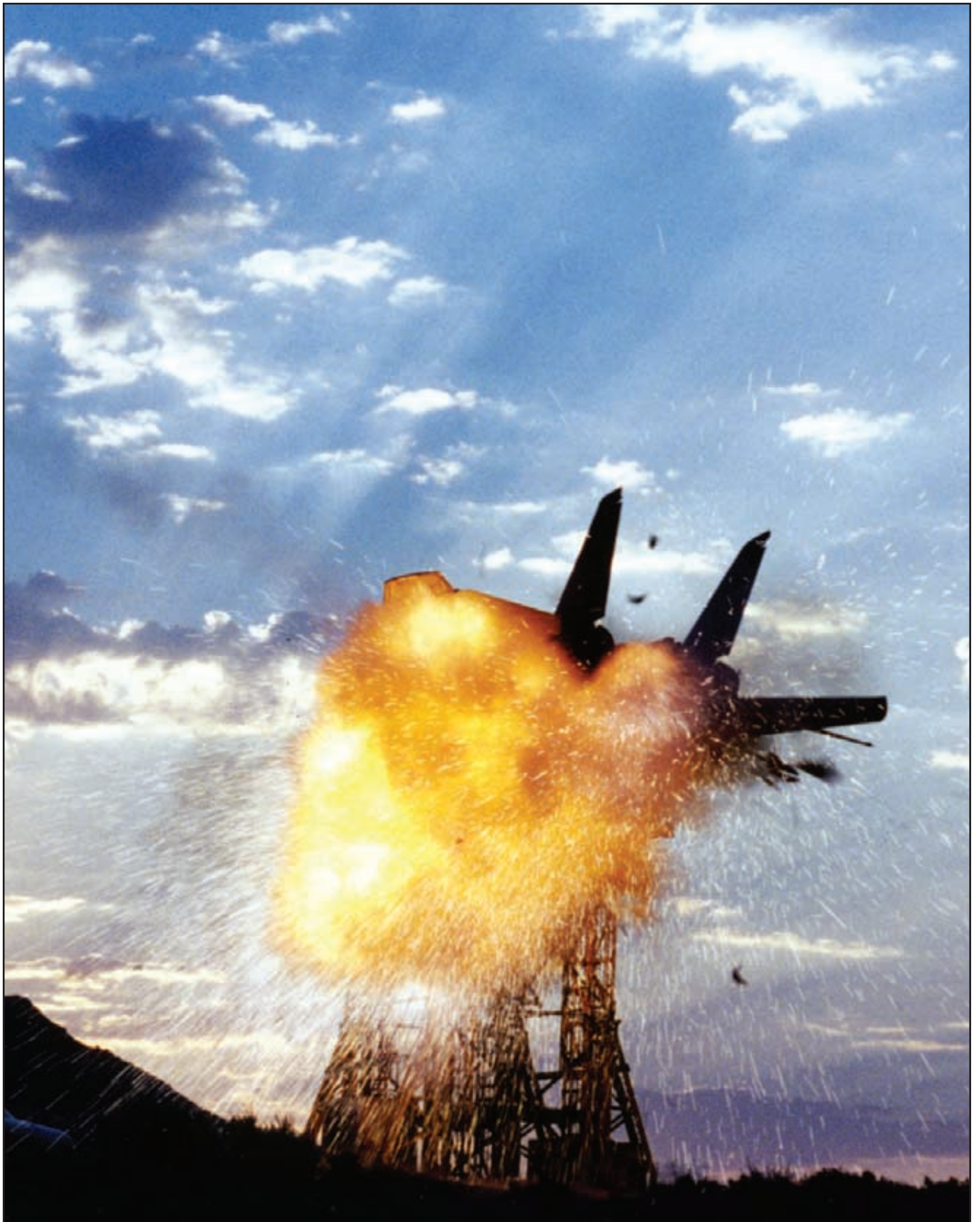
A Stinger Missile impacts an F-14 Tomcat test article just after sunrise on the Land Range.
