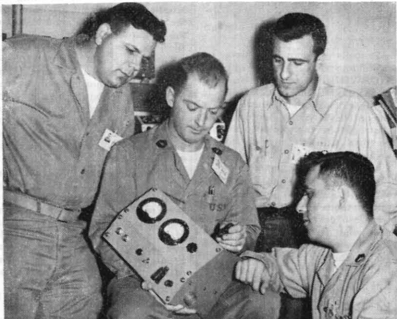
FIELD TEST EQUIPMENT —Military personnel work on a Field Test set which is used in testing the guidance and control section of the SIDEWINDER missile. Pictured (l. to r.) are: Chester Cannon, T/Sgt., USMC; Michael Wiczerzak, M/Sgt., USMC; Joseph Pillittere, GFAN, USN; and Thomas Moscoe, S/Sgt., USMC.
