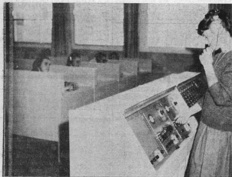
CONTROL PANEL —A student pinch hits for teacher in a demonstration of the mechanics of the control panel. The central switchboard permits communication between teacher and individual student stations.
