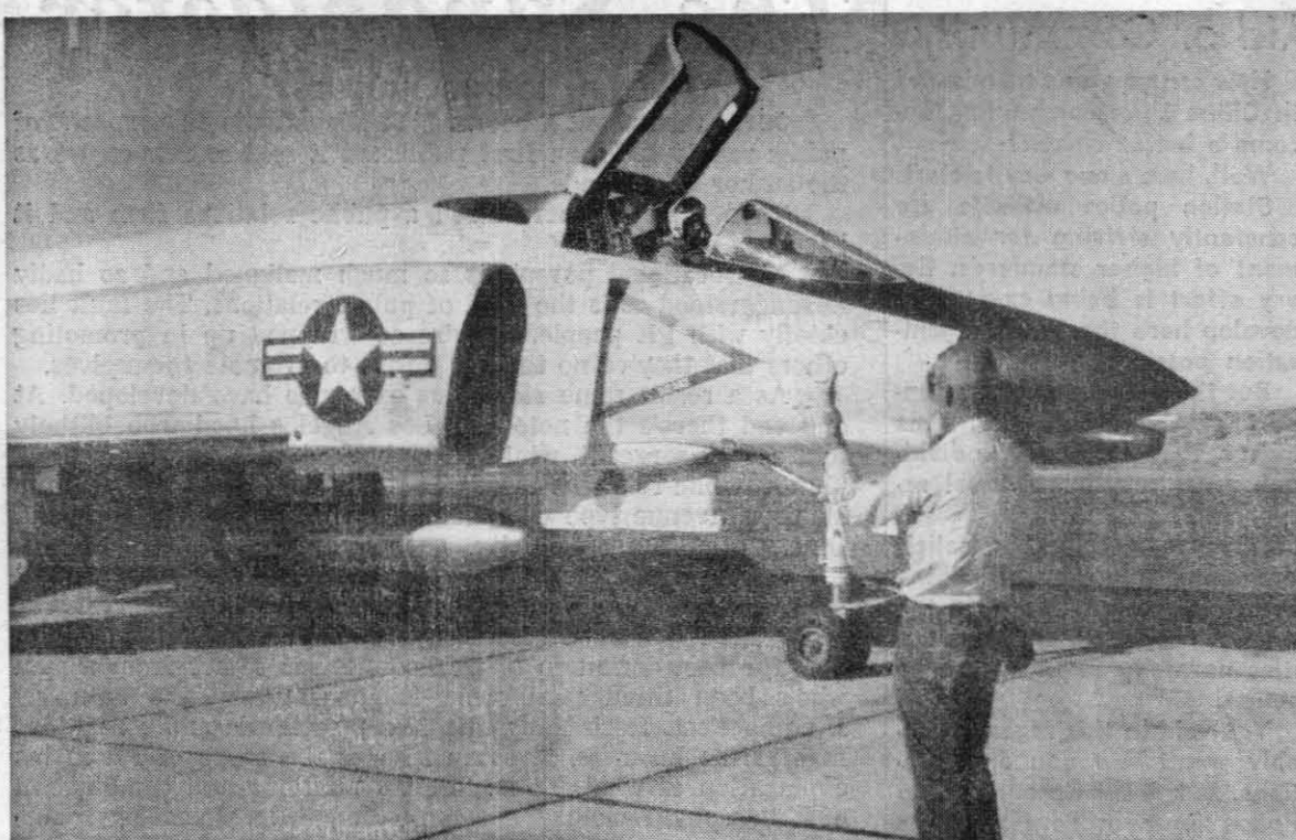
NAVAL AIR FACILITY'S F4H-II Phantom jet, piloted by LT Al S. Newman, moves down strip for takeoff with Caleb rocket slung under belly. Two-stage rocket hurt-
