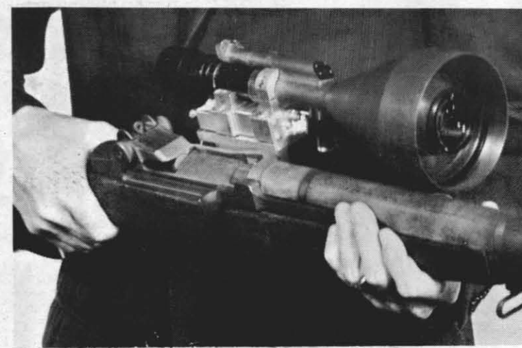
BUSINESS END OF LASER rangefinding sniper scope is shown, with its lens within a lens (see story). Designer Ted Bergman hopes to have prototype ready to fire this year.
