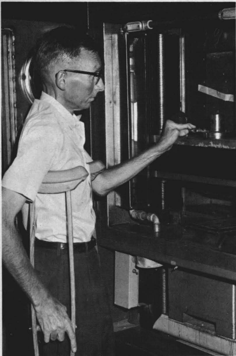
KEN BISCHEL PREPARES for testing a solid propellant structure in the Instron tensile tester at the Pilot Plant. Ken is a research chemical engineer with Code 45, and works with local Boy Scouts. To combat effects of his progressive arthritis, he swims with the Draggin' Dolphins club twice a week in Station Pool.
