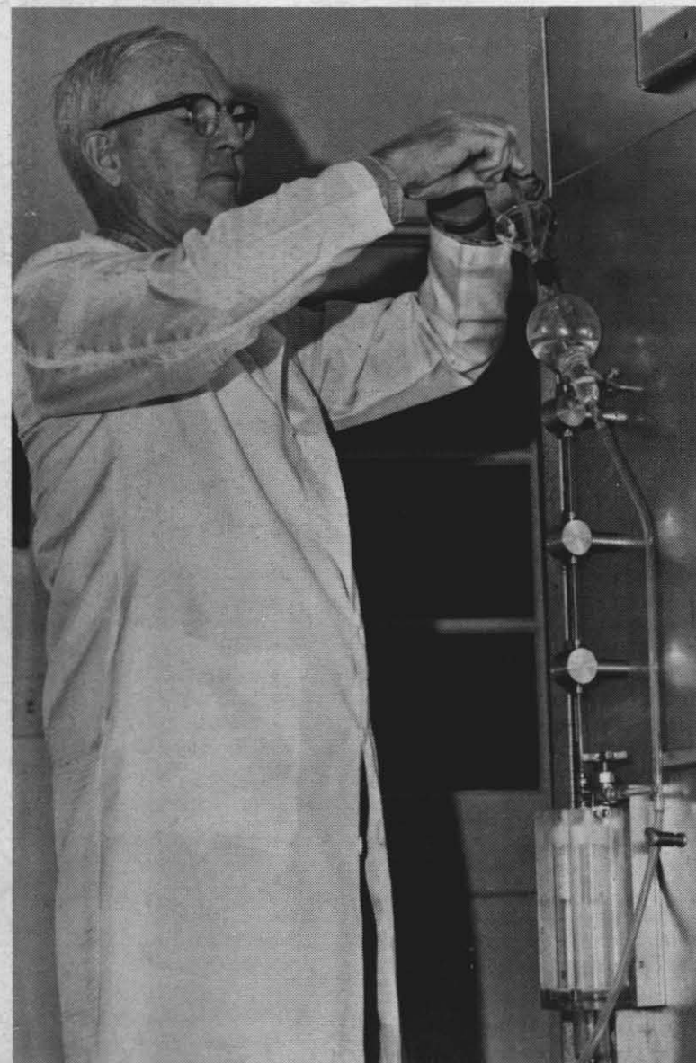
H. I. SCRIBNER, retiring from his NOTS career, performs a test on the "HYDRAT" machine which is used for measuring drag reducing properties of various materials.
