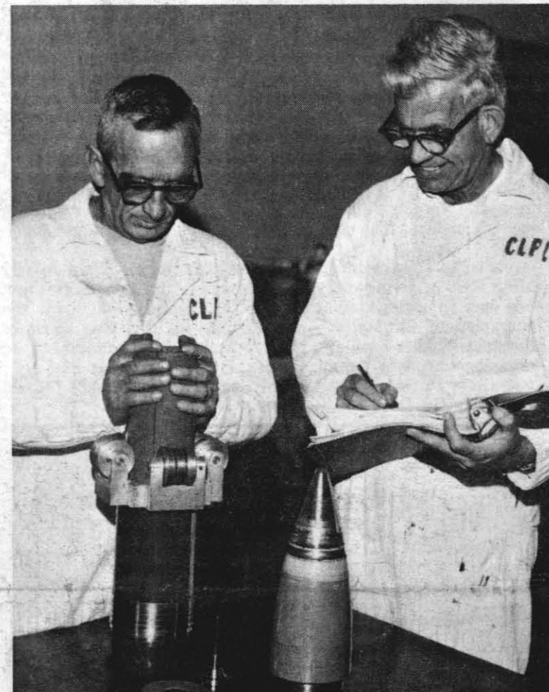
LOADING A RAP — Ordnanceman W. H. Smith loads propellant into a RAP round under the eyes of Bill Koch, mechanical engineering technician. Fuel and motor easily take 18,000 G's of 5-inch gun launch, plus 12,000 G's of spin through the rifling. High-impulse fuel burns for about two seconds, 23 seconds after launch. Howard Payne of Code 4573 is project engineer for motor.
