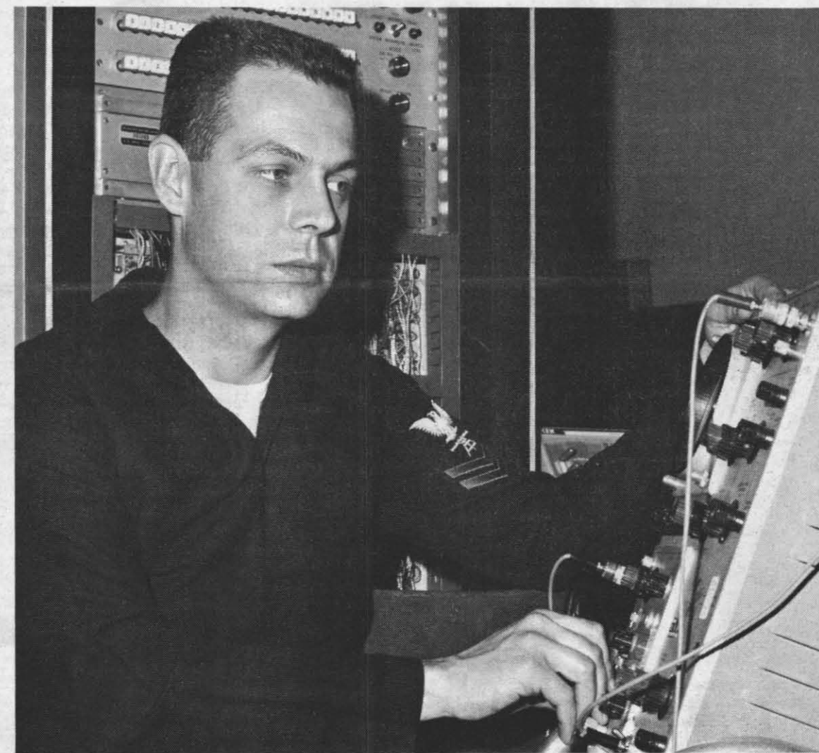
CHECKING HIS LOGIC — Bluejacket of the Month FTM-2 George C. Johnson works with a Navy Radar Building oscilloscope to check logic cards for the Digital to Analog Servo System (DASS). Johnson set off on
