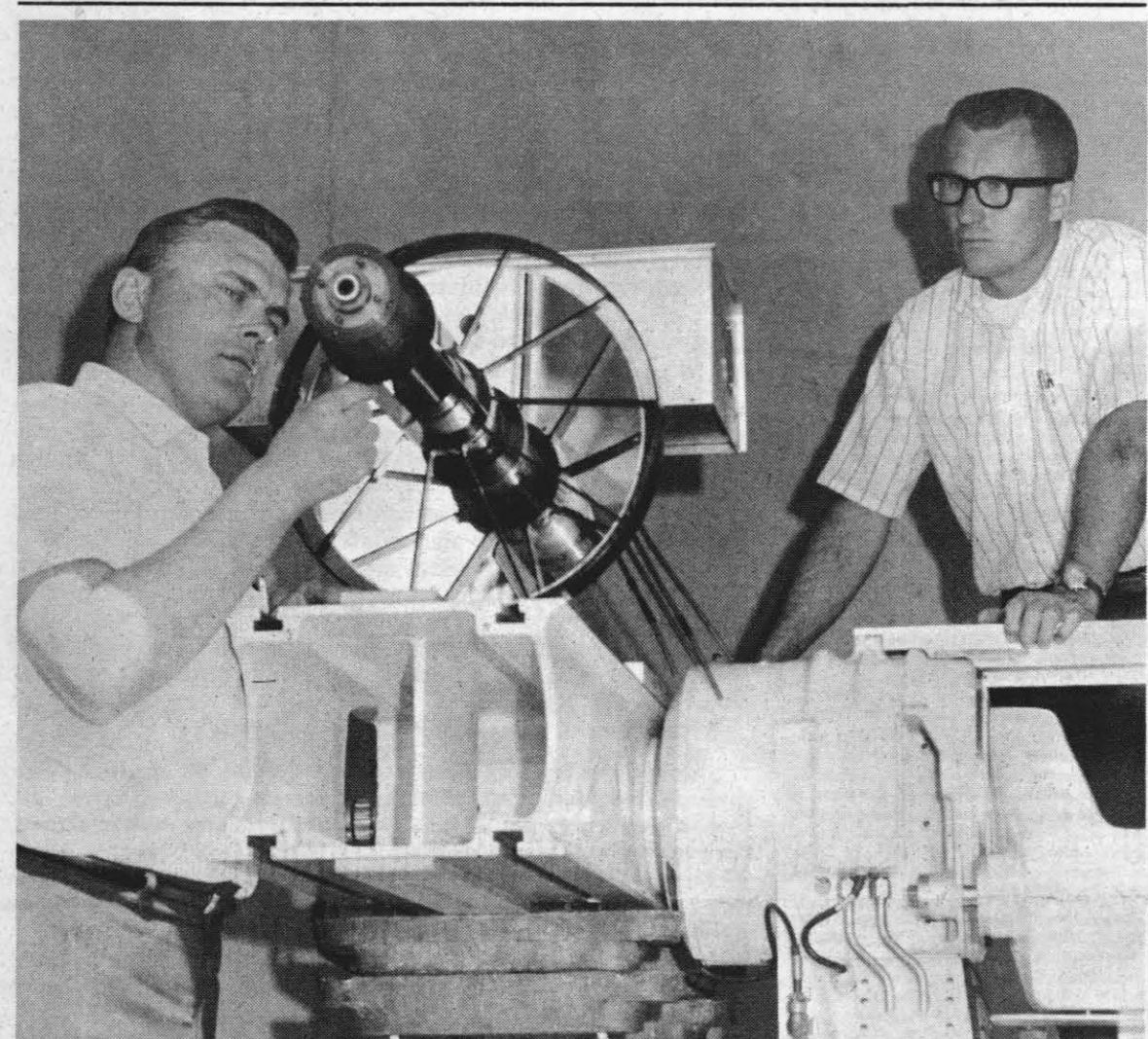
ONE-SITE SOLUTION BY LASER — Laser rangefinder project engineer Gary Kvammen checks receiver of laser unit mounted on new high-speed mount at Tower 11, G-2 Range. Harry Devereaux (right) is project engineer on mount. With tracking error detector device for elevation and azimuth data and to drive mount, entire system will be called Automatic Cinetheodolite, a "first" for Naval Weapons Center.
