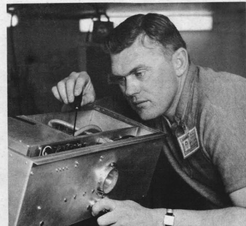
FINE ADJUSTMENT — Physicist Gary Kvammen makes small adjustment in laser rangefinder's new transmitter, which features a fast "Q-switch" providing for fast rise in each laser pulse to its maximum. Transmitter uses a ruby rod, segmented for greater cooling.
