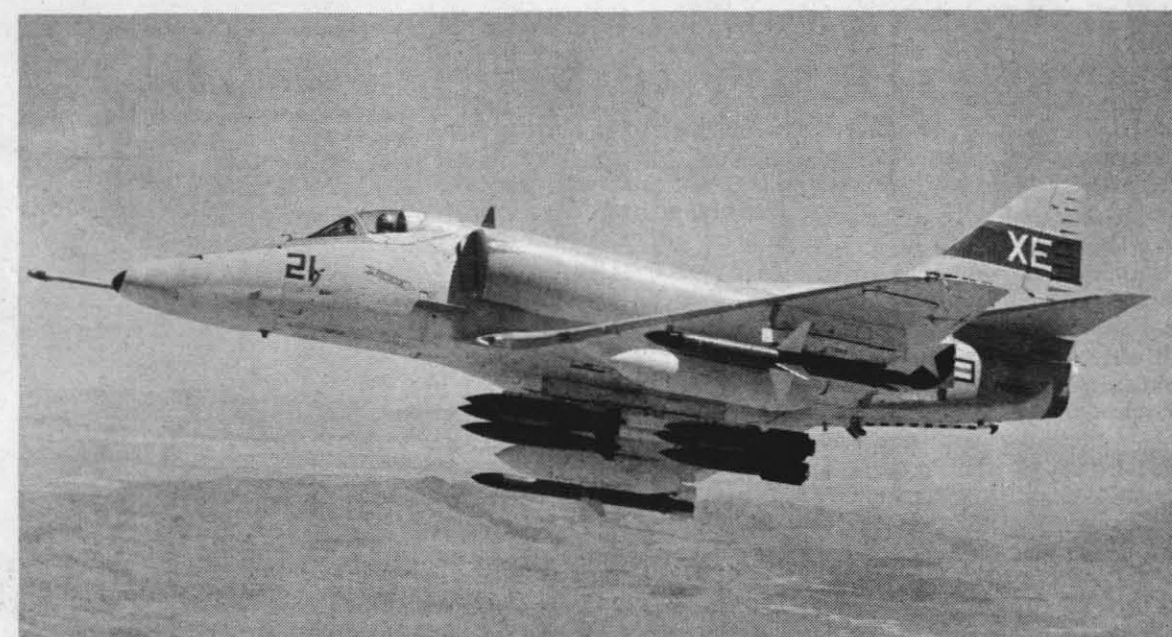
OTHER ORDNANCE — A variety of ordnance is carried on VX-5 aircraft such as this A4E with Shrike, 2.75 rocket pods and MK-81 250 lb. bombs.
