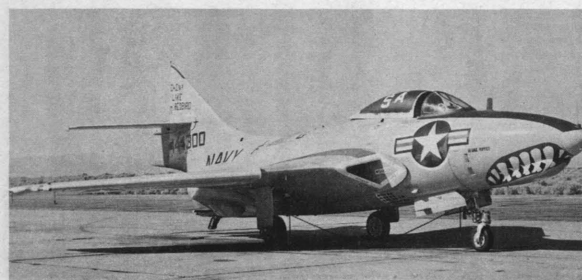
SNARLING "REDBIRD" —This is one of the pilotless reddish orange F-9 jet drone aircraft that are flown by remote control by a pilot in another aircraft.
