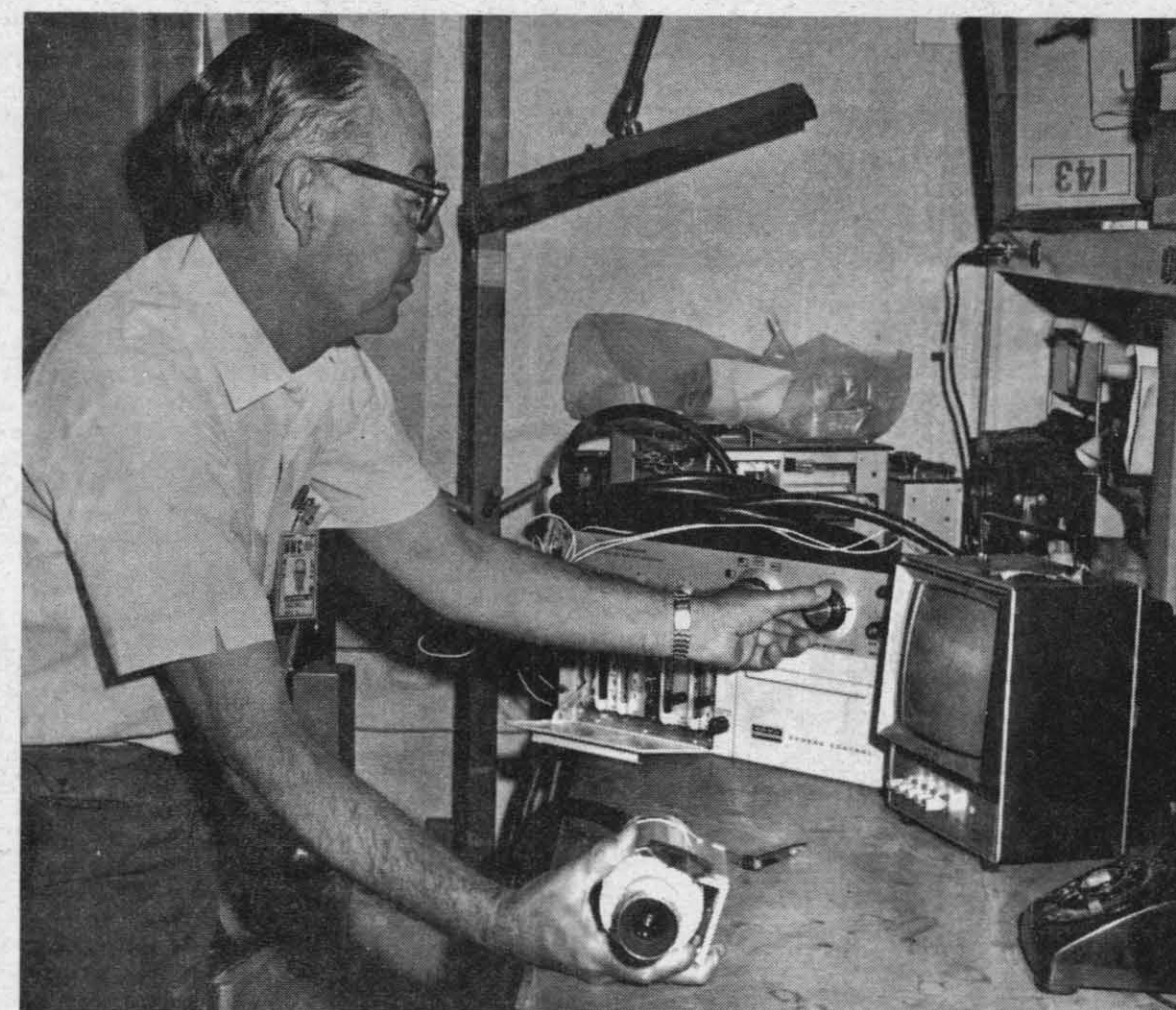
VIDEO CAMERAS mounted in Project Stormfury aircraft will be monitored on a television receiver capable of producing a split-screen image. This effect is made possible through the use of a special effects generator. Neil Waggoner, Airborne Instrumentation Branch, AOD, is shown checking out the equipment and its components in Hangar No. 3 at the Naval Air Facility. NWC has also been responsible for the development and installation of much of the meteorological instrumentation used on Hurricane Hunter aircraft. —Photo by PH2 Kenneth Stephens
