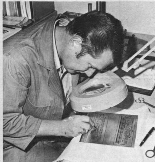
**TOUCH UP**—Minor pinholes and imperfections are covered with an etch resistant ink prior to etching. Charles Knowles is shown touching up a circuit that has been treated with a dye to make imperfections visible under magnification.
