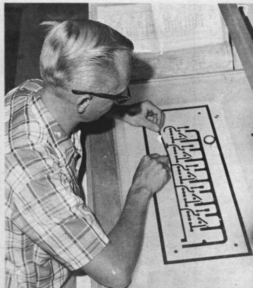
**ARTWORK LAYOUT**—Roger McCollough, Electronic Technician, is shown taping master artwork of a printed circuit layout. The artwork will be photographically reduced to actual size and a film mask made up for use in the printed circuit process.
