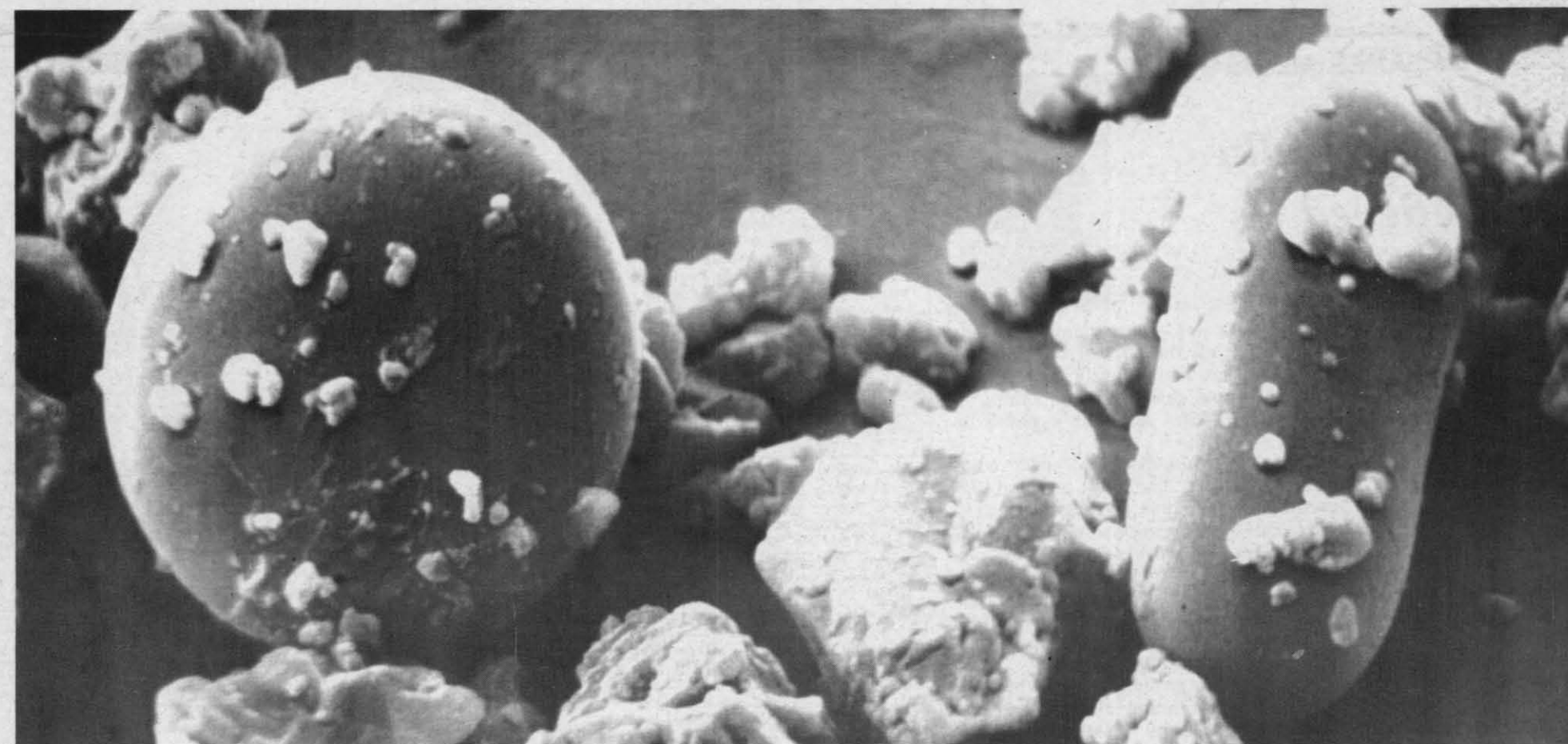
A SAMPLE OF LUNAR DUST as seen under 4000X magnification is revealed to be a collection of microscopic glass beads and pieces of shattered crystalline material (large rock-like objects) that have been formed over the years from lunar basalts. The large oblong shape on the right and the round object on the left were found to be common shapes. According to investigators, they
