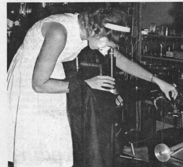
JEAN BENNETT make a final wavelength setting while measuring the thickness of a very thin evaporated film. These interferometric measurements are made using the so-called fringes of equal chromatic order and are an extremely accurate method of measuring very small thicknesses.
