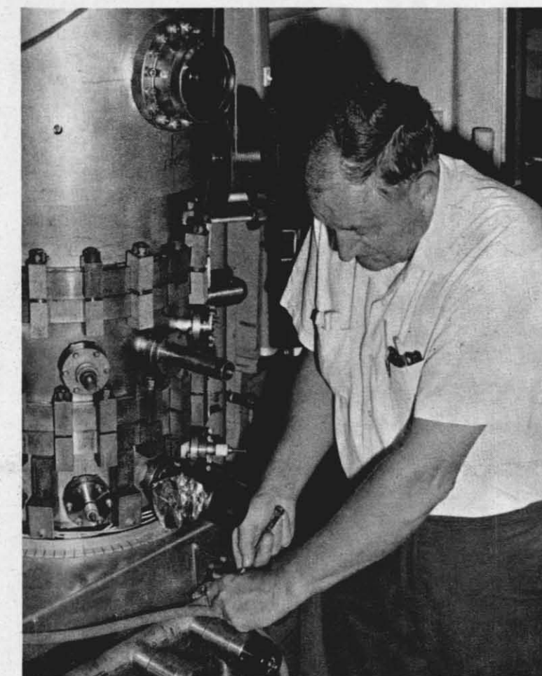
ED ASHLEY is finishing replacing the pump on the ultra-high vacuum evaporation tank. With this system, very pure materials can be prepared on which to make precision optical and electrical measurements.
