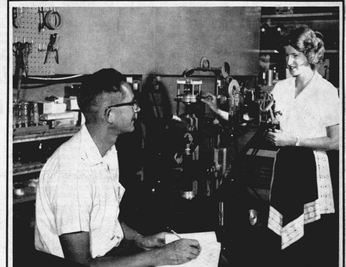
JEAN BENNETT make a final wavelength setting while measuring the thickness of a very thin evaporated film. These interferometric measurements are made using the so-called fringes of equal chromatic order and are an extremely accurate method of measuring very small thicknesses.
