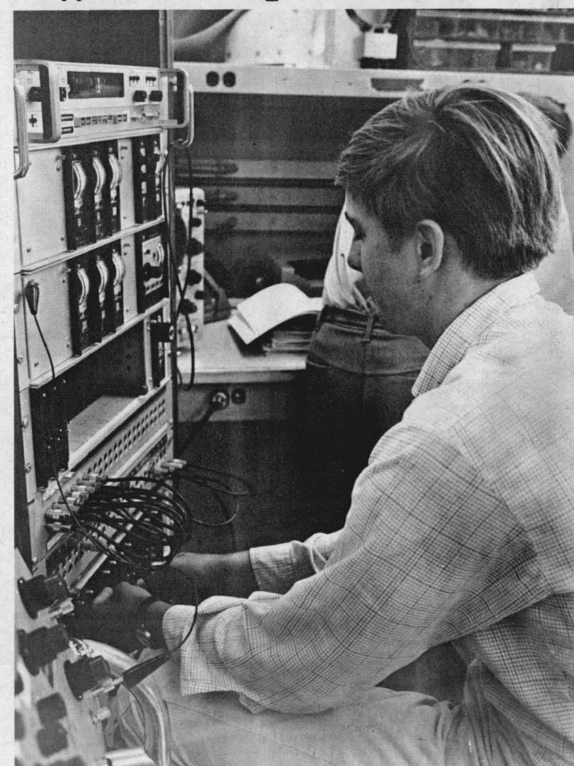
ABOVE — TOM RAFALSKI is an engineering aide from Bakersfield College where he is an electronics student who plans to enter Electrical Engineering. Here Tom works at tuning F.M. multiplex equipment for Code 4056.
