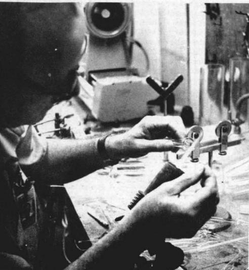
**ABOVE, RIGHT**—Griffith is seen working on another inner part of an AGILE detector package. Here the metal leads are being set in the glass to make the electrical connections for the detector, which will be mounted inside the glass. **RIGHT**—The Code 60 glassblower is seen working with one of the basic forms of many blown glass art forms. This is the body of a swan.
