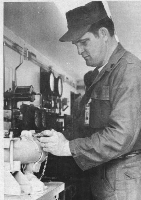
**VITAL STEP PERFORMED** — SSgt. R. F. Garrett, one of two Marine staff NCOs trained to operate the missile maintenance van, practices one of the key operations—recharging of the Sidewinder launcher gas receiver.
