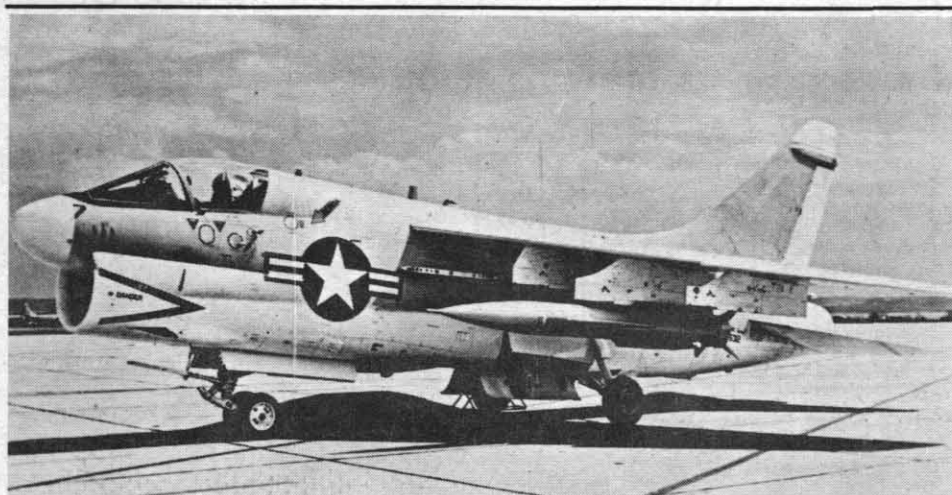
MILESTONE MARKED IN TEST PROGRAM — The Air-Launched Low Volume Ramjet test vehicle, shown in a pod carried below the wing of an A-7 Corsair II, met or exceeded all requirements recently during its first free flight range test. The test was carried out over the Naval Missile Test Center's Pacific Missile Range.
