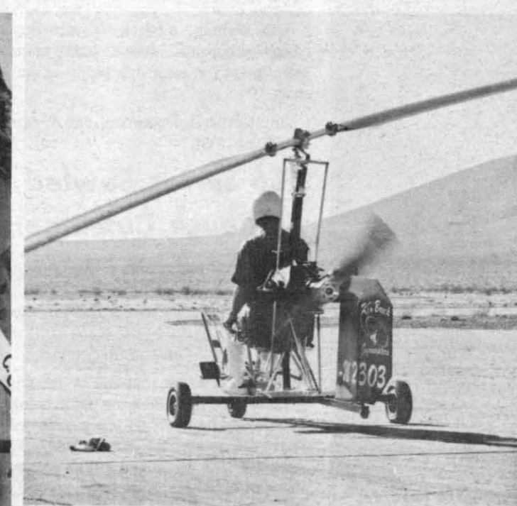
FIRST-TIME ATTENDEES at the air show were probably surprised to learn that the Benson gyrocopter, piloted by Ken Brock, gets all of its power from the small engine mounted at the rear. The rotors which spin and lift the tiny aircraft as it gains forward speed from the power plant are not connected to the engine.
