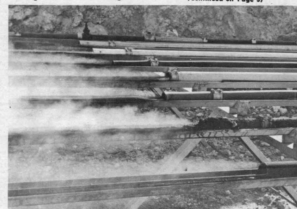
TWO METHODS OF CORROSION STUDIED — A test array, located at Devil's Kitchen, shows the two different forms of geothermal corrosion being studied by a group led by Dr. Carl Austin, head of the Research Department's Petrodynamics Branch. Half of the pipes are used to study corrosion in an anaerobic (no air available) state, while a split pipe, leaving a U-shaped conduit, is aerated, allowing test engineers to study corrosion in a complete sequence from air being mixed with fluid to a point where oxidation builds up. —Photo by Tom Carter
