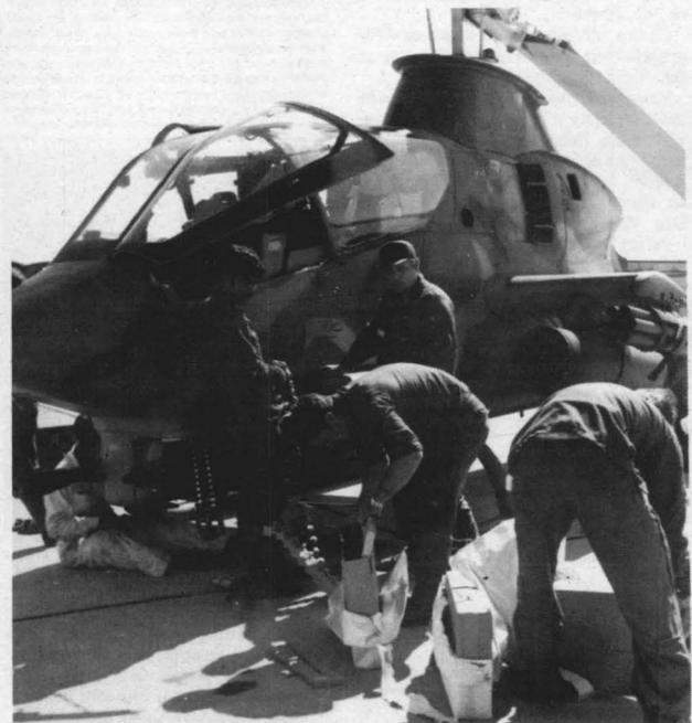
WEAPONS LOADED FOR FIRING TESTS — Personnel from the Army's 155th Aviation Company are shown loading 40mm guns in preparation for extremely low level firing runs by AH1G Cobra helicopters at the Airport Lake range. In addition to the 40mm guns, the helicopter pilots also fired 2.75 in. folding fin aerial rockets and 7.62mm machine guns.
