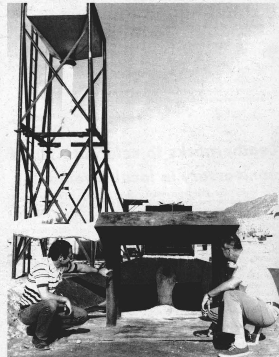
IMPRESSIVE STRUCTURE — At T range's airflow facility, Tony San Miguel (at left) and Tom Horeff inspect the propane torch under the airfoil used to ignite fuel during testing. The partially-obscured grill is the exit plane of the diffuser. The 18-ft. high tower at left is the fuel hopper used to pour the fuel into the airstream.
