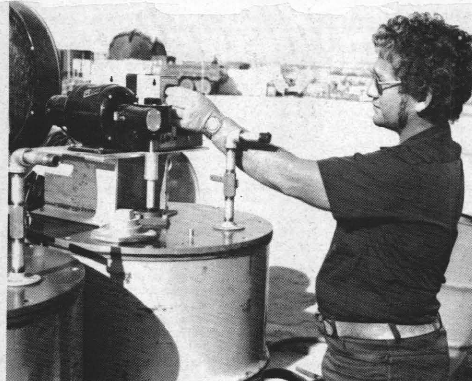
DELICATE WORK — Marion "Willie" Williams, a mechanical engineering technician for the Fire Program Office, is shown adjusting the pilot plant apparatus for mixing an antimisting agent with Jet-A fuel, a commercial kerosene. The mixing process is very critical to the additive's effectiveness.
