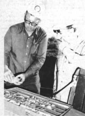
**DRILL SAMPLE STUDIED** — Dr. Peter Waterman examines a sample of hydrothermally altered drill core that is being shown to him by Dr. Carl Austin. Steam and hot water have penetrated through fractures in underground rock to create new chemical compounds from the original host rock.
