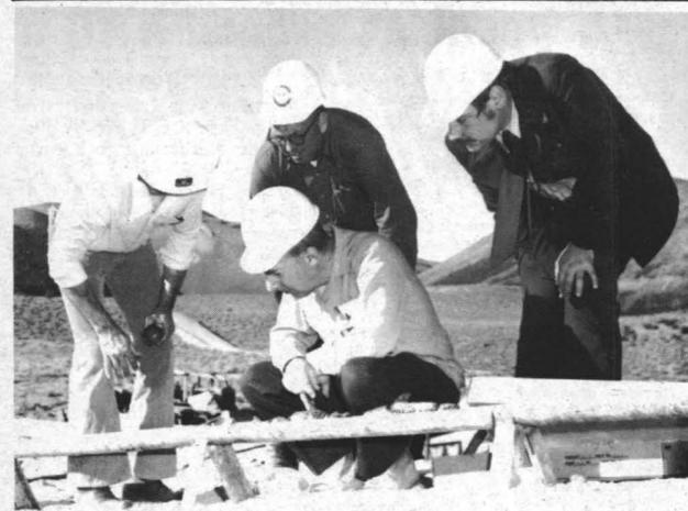
**CLOSE LOOK TAKEN AT DRILLING CORE** — Dr. Peter Waterman (kneeling) looks over a section of the wire-line drilling core, noting the alterations that have taken place in it after being exposed to steam and hot water in the superheated hot dry rocks underground at the Coso geothermal area. Others in photo are (from left) Walter Adams, Dr. Carl Austin and Peter Ritzcovan.
