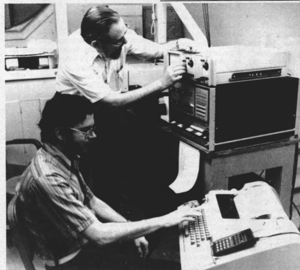
NEW INVESTIGATIVE TOOL — A fast Fourier transform interferometer spectrometer has been developed by employees of the Propulsion Development Department's Applied Sciences Branch. It provides a new and unique measurement capability for investigation of the infrared spectra. Shown demonstrating how it works are Dr. Mel Nadler, seated at the teletype that feeds instructions to a computer, and Bob Blunt, who is adjusting a knob on the display monitor. —Photo by Ron Allen
