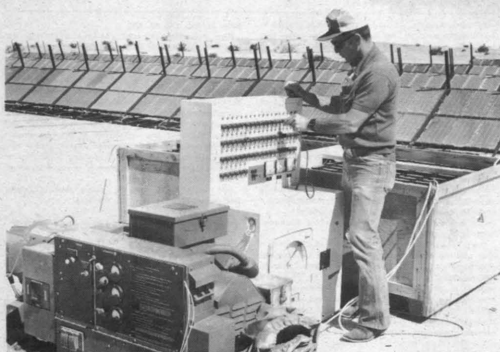
CHECK-OUT-MADE — Ralph Brewer, an electronic technician in Code 3153, checks the output of the photovoltaic panels (arrayed in the background) with a test console. The batteries, still partly crated, are shown to the right of Brewer and behind the test console. They weigh approximately one ton each. At left is the motor generator which powers the radar.
