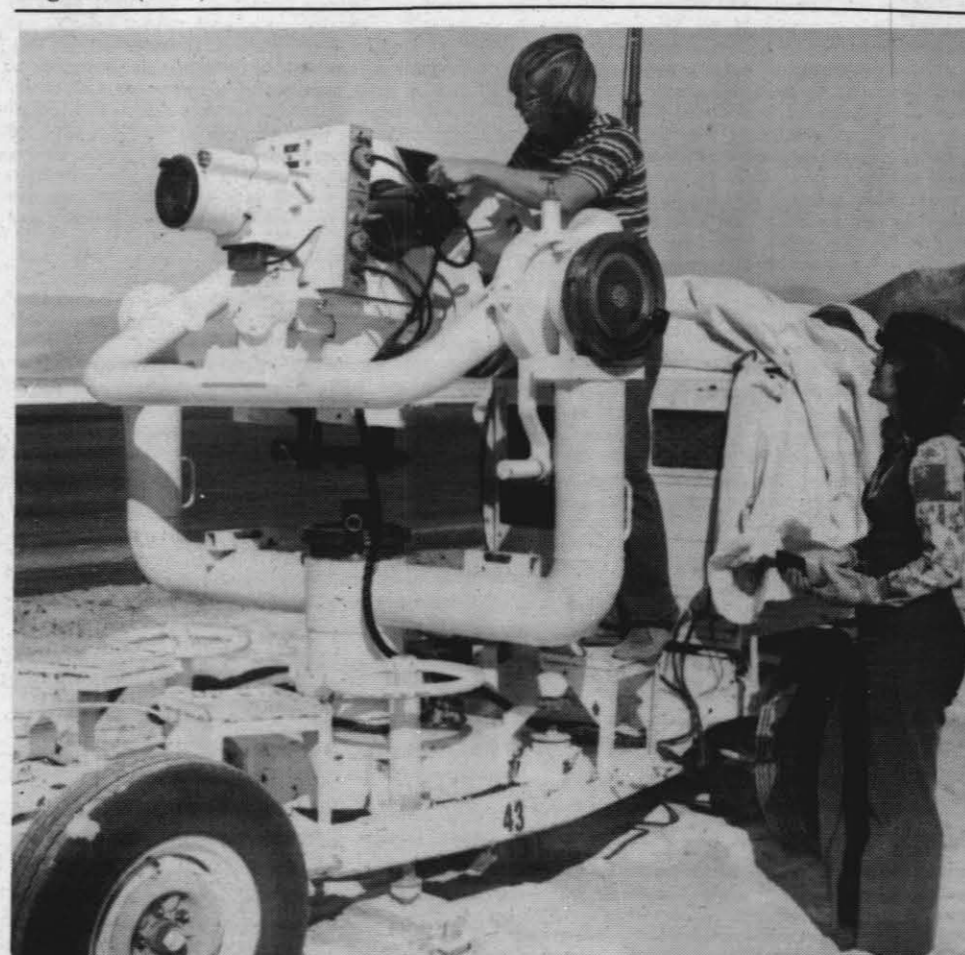
LOCAL PRODUCT — Robert G. Hams, a test range tracker for the Air Operations Branch of Code 62, sets the frame rate and exposure of the CZR-1 Bowen camera system, while Mrs. Margaret A. Chandler, also a Code 62 tracker, looks on during an operation at G Range.
