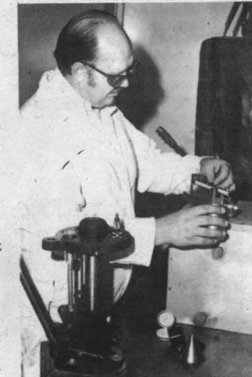
METICULOUS WORK — Robert Gould, an aerospace engineer in Code 3244, is working in the Ordnance Systems Department's Shotgun Facility loading ammunition for propellant evaluation. Shotgun shells, filled with a solid propellant, are fired at a steel plate, and fragments of the propellant are caught in a basket.
