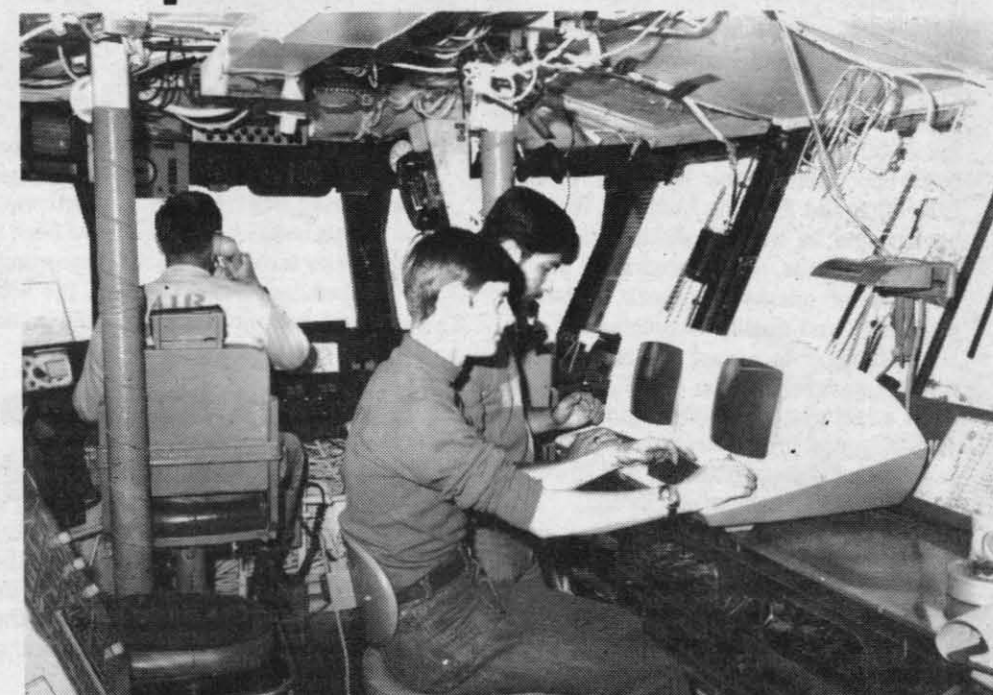
EYES OF THE AIR CONTROLLERS — Five decks above the Kitty Hawk's flight deck, in the primary flight control room (or tower), Cdr. Robert Harshbarger, the ship's air boss, directs the recovery of aircraft while ABH3 Bob Vish (in background) and ABH2 Tom Sharnak enter data on the room's two LINDA consoles. The air controllers themselves are "buried" below decks and cannot see the aircraft they are directing; the personnel in the flight control room are the only ones who can see the aircraft and deck situation for this purpose.
