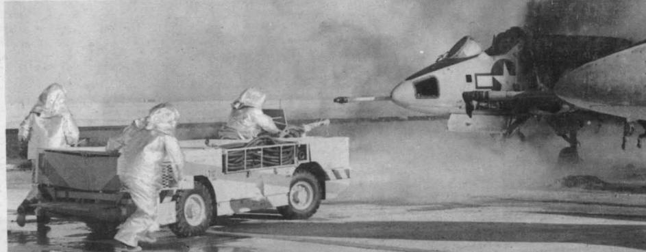
READY FOR ACTION — The P-16 aircraft carrier fire-fighting vehicle swings into position at the mini-deck area at NWC's Aircraft Survivability Range. Surplus aircraft used for these tests, while no longer flyable, still provide the needed elements of realism since they are parked in the same way that aircraft would be located on an actual carrier deck. —Photos by Ron Allen
