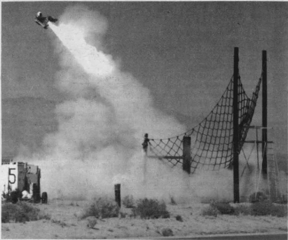
UP AND AWAY! — The seat and dummy soar skyward after ejection from the sled-mounted A-6 aircraft cockpit. This zero-altitude, zero-speed test demonstrated the stability of the vertical-seeking aircrew escape system. Further tests planned will demonstrate the system's capability to achieve a vertical-up trajectory when ejection takes place from either a banked or an inverted cockpit.
