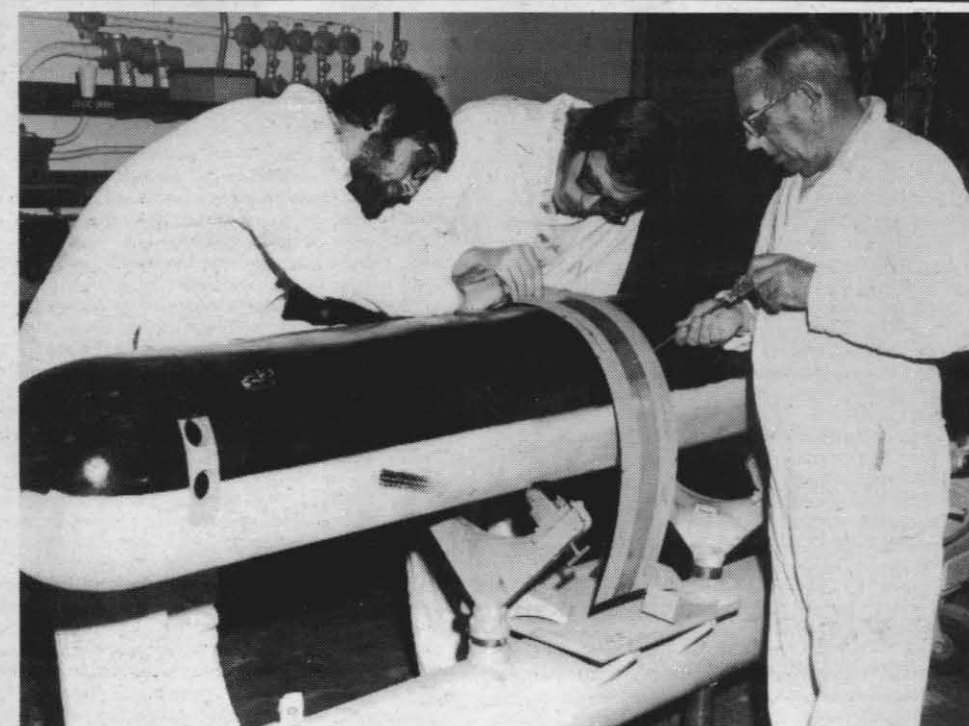
ANTENNA INSTALLED — NWC Vertical Launch Prototype Demonstration Program personnel install a wrap around antenna on the ASROC missile that was successfully launched from the vertical launcher. They are (l. to r.) Scott O'Neil, Mike Ripley and Bob Willard of the Systems Technology Branch. Ripley is the program's project engineer. —Photo by Ron Allen
