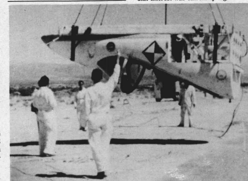
ON THE MARK — The SNORT crew prepares to hoist the vertical-seeking seat test hardware into position 100 feet above the ground.
