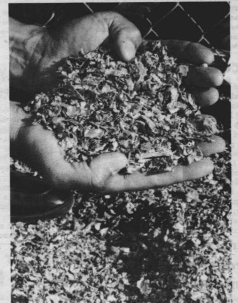
**CONDENSED CANS** — The aluminum cans collected are shredded, both for ease in shipment and for higher resale value. Recycling of cans represents a major saving of energy: processing one pound of new aluminum requires 8 kilowatt hours of electricity (the energy equivalent of 5 pints of crude oil), while reprocessing a pound of aluminum requires only 5 percent of the same amount of energy.
