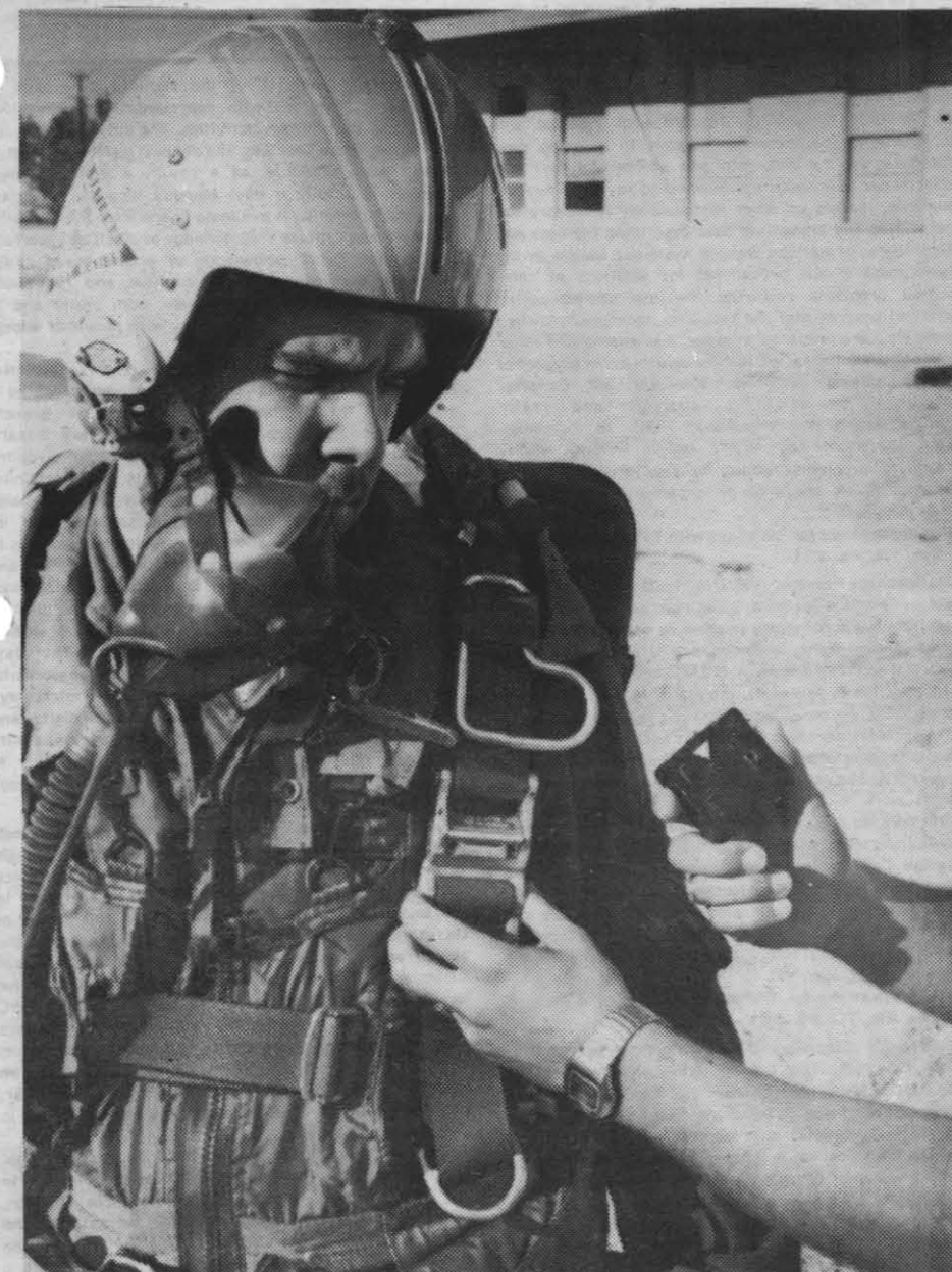
TEST GEAR EXAMINED — PRAN Cliff Mathews is suited up and ready for a test of a proposed automatic parachute divestment system. One of the main components of his system is the device held at right that is to be adapted to the parachute canopy release fitting.
