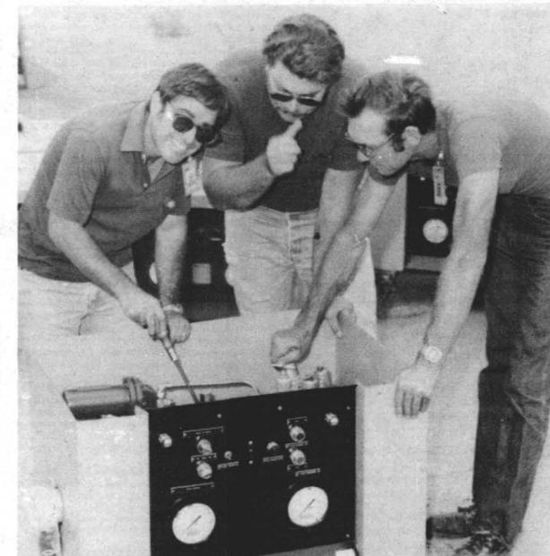
**SIZABLE SAVINGS REALIZED** — From old equipment destined for the scrap pile at NATC, Patuxent River, Md., employees of the Public Works Department Machine Shop cannibalized parts used in fabricating "like-new" compressed air consoles for use in starting up jet aircraft engines. The savings, compared to the cost of purchasing such equipment new, was estimated at \$250,000. Shown checking over one of the consoles are (l.-r.) equipment mechanics Frank Henzel, Rodney Nyholm and Ed Duff.
