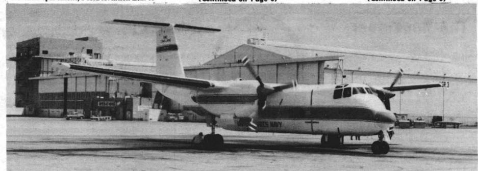
**ALL SPRUCED UP**—The Center's DeHavilland C-8A Buffalo's gleaming blue and white exterior is representative of its complete overhaul, which has just been completed. The aircraft will serve as a platform for parachutists and will also be used for transporting personnel cargo. Refurbishing the aircraft saved \$13 million since a new Buffalo costs \$14 million.
