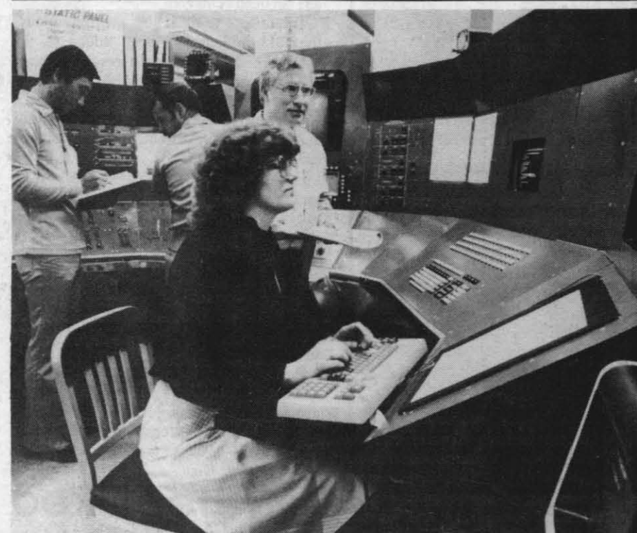
SIMULATED FLIGHT — Hard at work in the F-18 Weapon System Support Facility (WSSF) are (l. to r.) Jim Takahashi, Cdr. J. P. Connell, and Cliff Ransom, as Fiona Nave sits at the computer. The WSSF is a computer simulation laboratory used for development, verification and validation of software needed by the F-18 Hornet.
