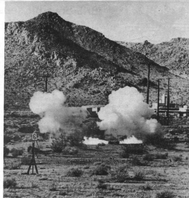
DRAMATIC DISPLAY — The burning of an ASCROC shell grain N-5 propellant shows what could happen in a premature ignition. In the foreground is the frame of a dummy "ordnanceman," all that is left after a one-gallon container of R-98 propellant was ignited nearby.
