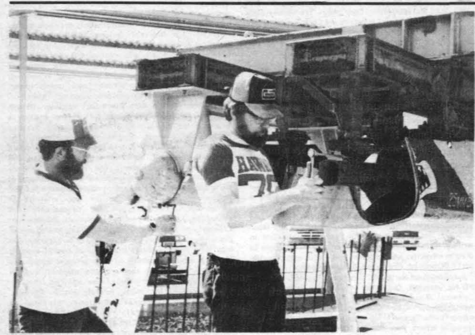
GUN PREPARED FOR AMMO TESTS — Bill Glidden (at left) and Chuck Fowler, employees for the General Electric Co., check out the 25 mm GAU-12/U in preparation ammunition-firing tests at the Automatic Gun Bay of the Ballistic Test Range.
