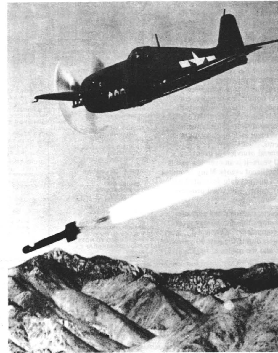
TINY TIM, an 11.75-inch torpede-shaped rocket developed during World War II, is fired over China Lake ranges during 1944. Operations were conducted from Harvey Field (now the Inyokern Airport) before air units moved to Armitage Airfield. Tiny Tim weighed 1,250 lbs.
