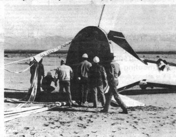
**LOOK INSIDE** — Several personnel from the Aerosystems Department and others involved with the Space Shuttle booster program take the opportunity to peer within the drop test vehicle that was used to simulate the booster in parachute tests.
