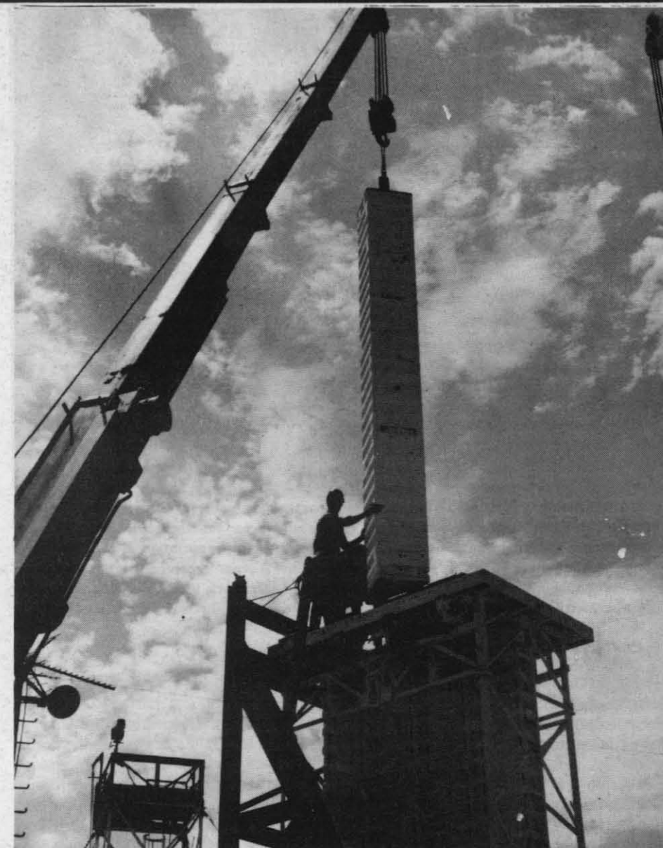
LOADING — A rigger carefully guides the cannister into the appropriate module for the Vertical Launch ASROC test held recently.
