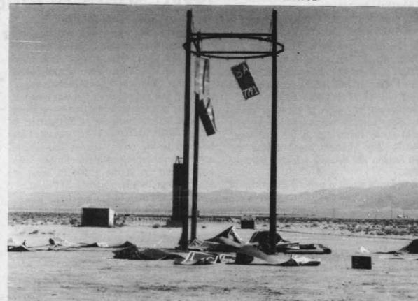
**AFTERMATH** — Witness plates scattered around the test structure show the effects of a warhead blast.
