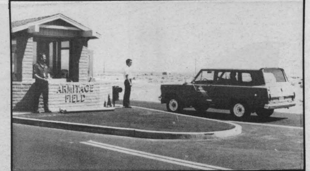
INVISIBLE DRIVER? — The gate guard to Armitage Airfield does a double take as the driverless Department of Energy's Jeep Cherokee station wagon pauses at the airfield gate so the passenger can show his pass. Actual control of the vehicle is with the control box in the hands of Chuck Pierce, who is standing back of the guard.
