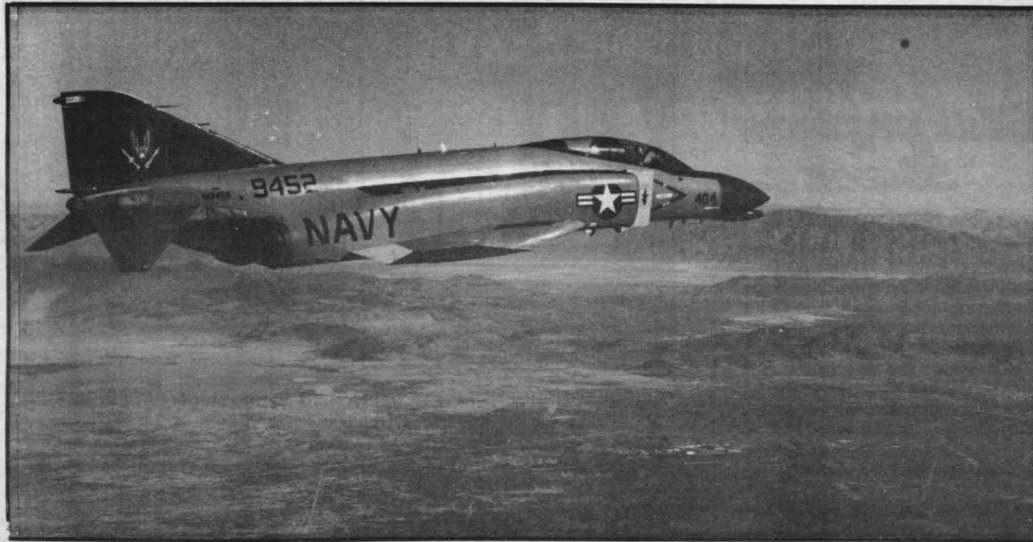
FIRST OF ITS KIND — A Phantom jet, newly converted to becoming a remotely piloted vehicle, zips through NWC skies in a test flight recently. The QF-4 is now
