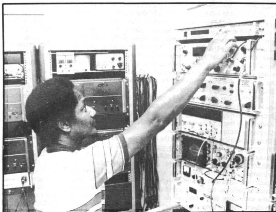
ANOTHER LEAP SECOND — Robert Cottingham, a member of the Metrology Engineering Section of the Metrology Branch, Code 3683, holds the button which retards the Center's atomic clock. Since 1958 this is the 22nd time that a leap second has been used to keep the atomic clock synchronized with the solar system and universal time.
