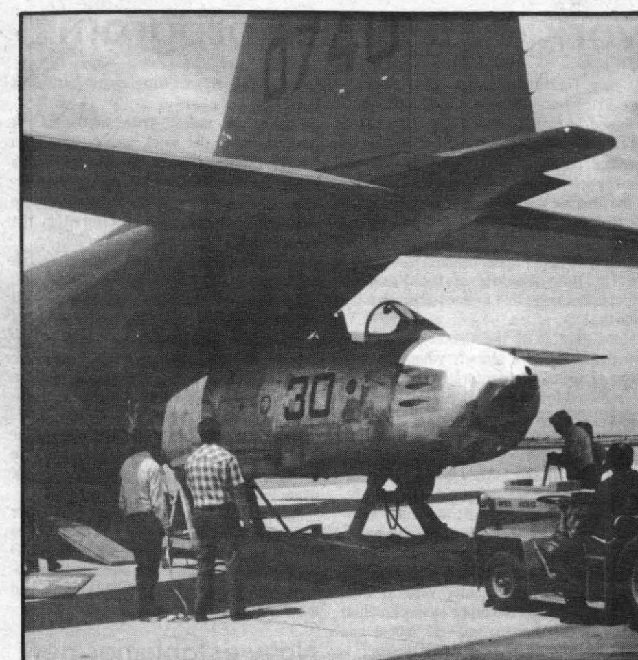
DISAPPEARING ACT — Soon to vanish into the vast cargo hold of a C-130 Hercules is the nose of a battle-damaged QF-86 target aircraft.
