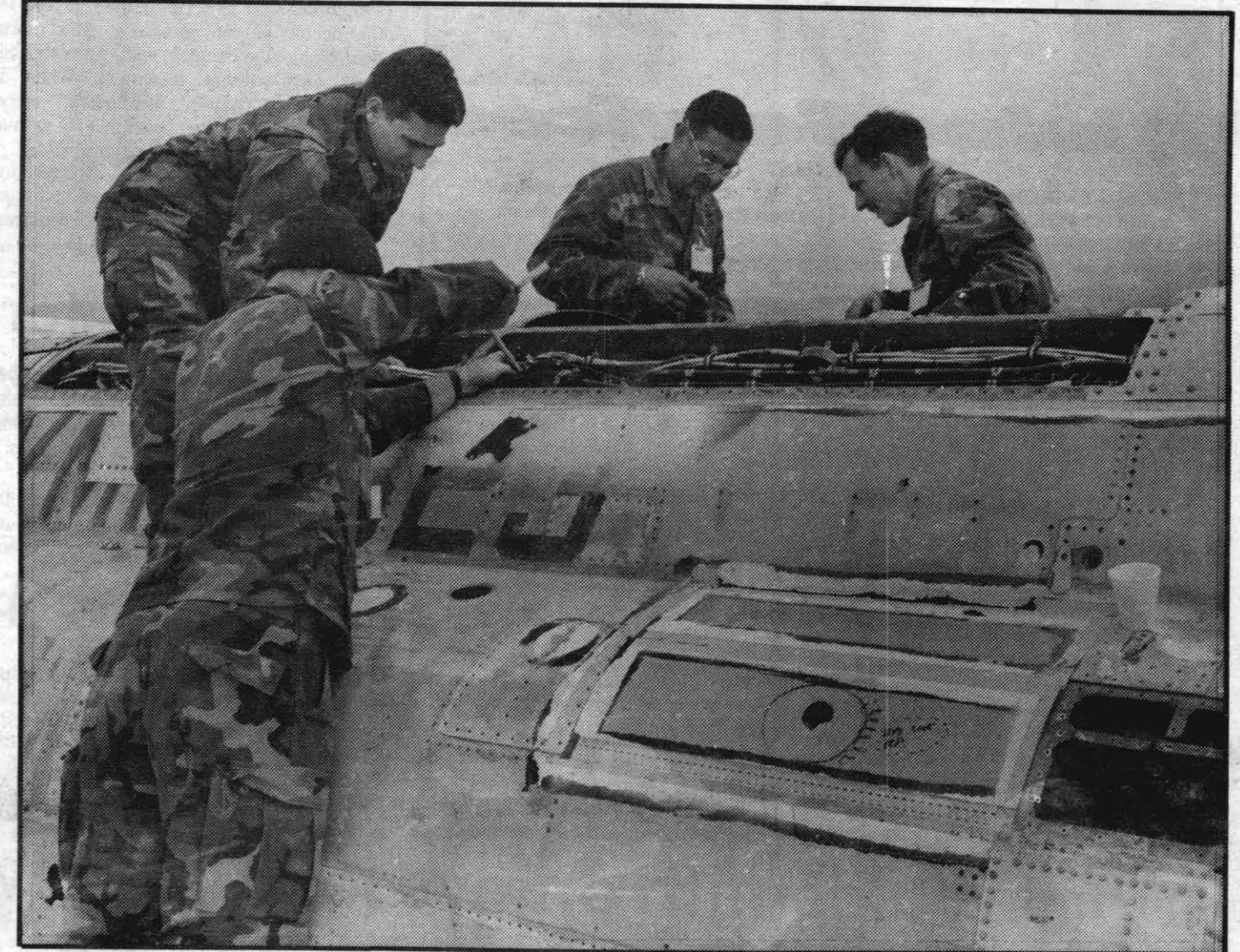
WORKING MARINES — Teaching fleet personnel how to repair battle damaged aircraft is the goal of the Aircraft Battle Damage Repair Program at NWC. Using
