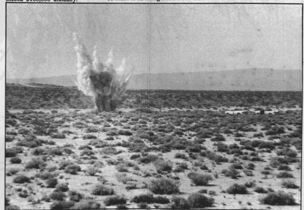
BANG! —Sound waves from the explosion are picked up by geophones and recorded by equipment in the two trucks. — Photo by Mickey Strang
